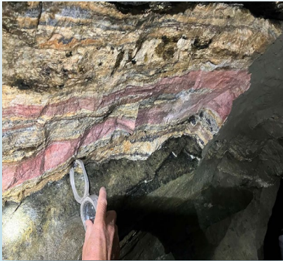
US Critical Materials Chief Geologist Peter Mejstrick taking a dip measurement of the exposed carbonatite. Approximately 4 feet of vein.
